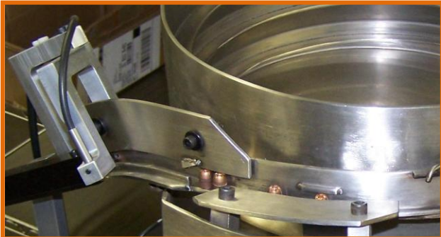
Rounds for the Air-Marshals are being feud into the final assemble machine.
